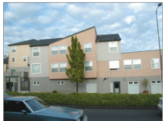
Inappropriate: Walls that appear “thin,” lack a sense of permanence, have a stage set appearance due to awkward proportions, lack articulation and use non-durable materials and bright wall colors
